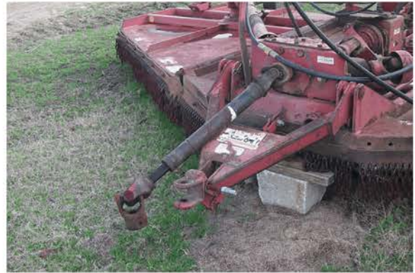
PTO driveline without safety guards.
