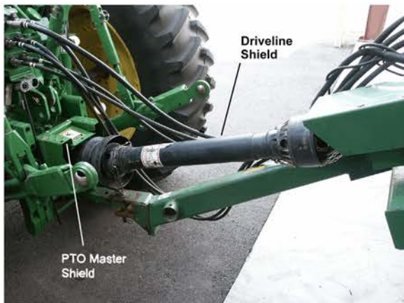
PTO driveline safety cover: All rotating parts are covered and the cover does not rotate.
